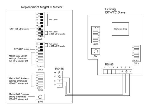
Figure 13 - Replacement MagVFC as Master in IST-VFC Compatibility Mode
