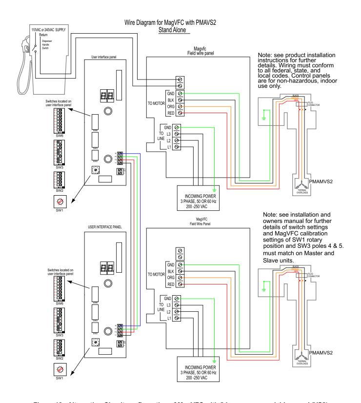
Figure 10 - Alternating Circuit configuration of MagVFC with 2 horsepower variable speed (VS2)
