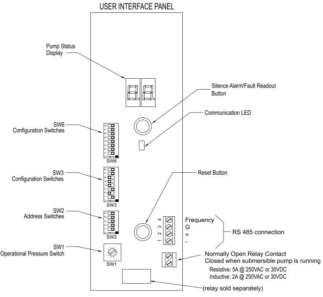
Figure 2: MagVFC Front Switch Panel
