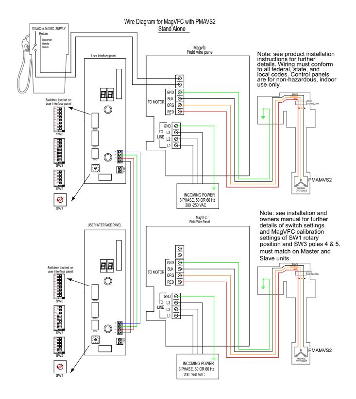
Figure 9 - Master/Slave configuration of MagVFC with 2 horsepower variable speed (VS2) (for connecting with VS4 pumps, turn SW3 Pole 6 ON for controller connected)
