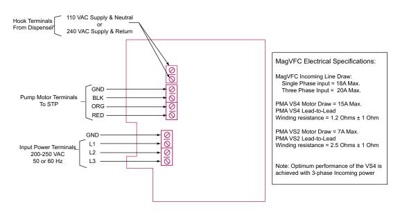
Figure 1: MagVFC Wiring
