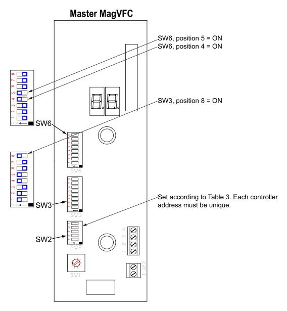
Figure 6: Switch Settings for Proportional Alternating Setup
