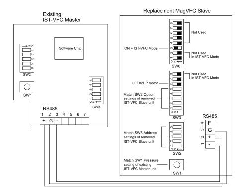
Figure 12 - Replacement MagVFC as Slave in IST-VFC Compatibility Mode
