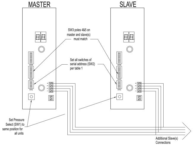
Figure 5: Setup Master/Slave Configuration
