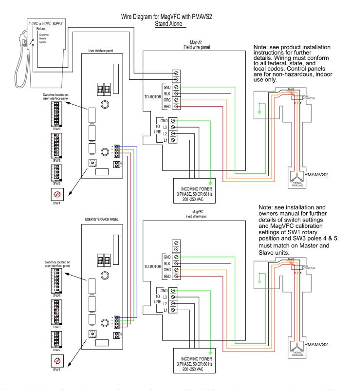
Figure 11 - Master/Slave-Alternating Circuit configuration of MagVFC with 2 horsepower variable speed (VS2) (for connecting with VS4 pumps, turn SW3 Pole 6 ON for controller connected)
