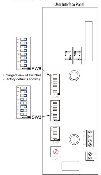
Figure 4: MagVFC Factory Switch Settings
