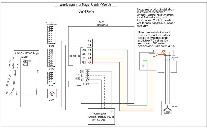
Figure 7 - Stand Alone configuration of MagVFC with 2 horsepower variable speed (VS2)
