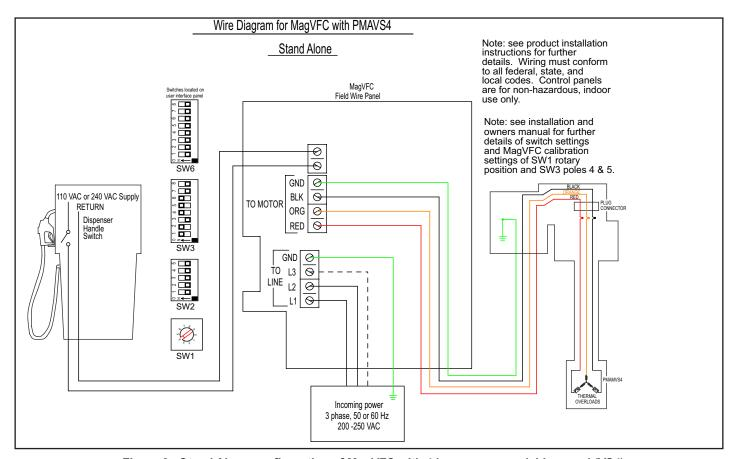
Figure 8 - Stand Alone configuration of MagVFC with 4 horsepower variable speed (VS4)
